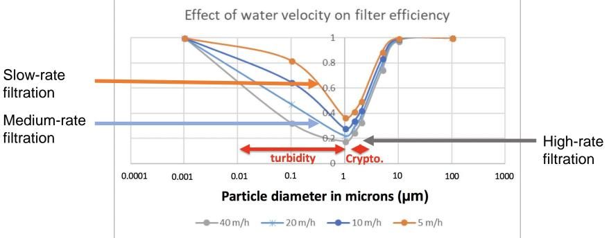
Filter efficiency is reduced as circulation rate is increased
